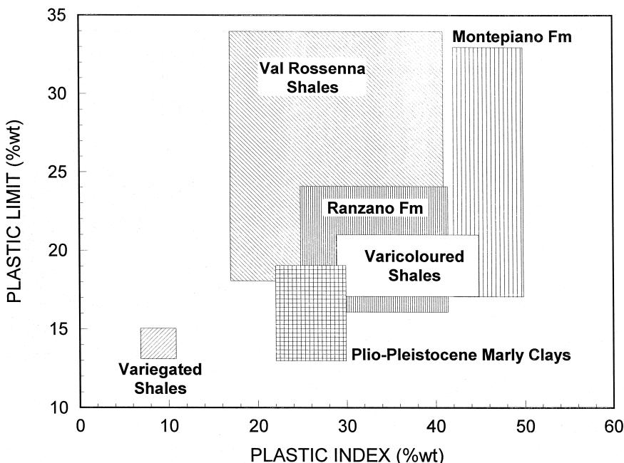
Fig. 9. Atterberg plastic index versus plastic limit of clay materials from the Sassuolo District.
