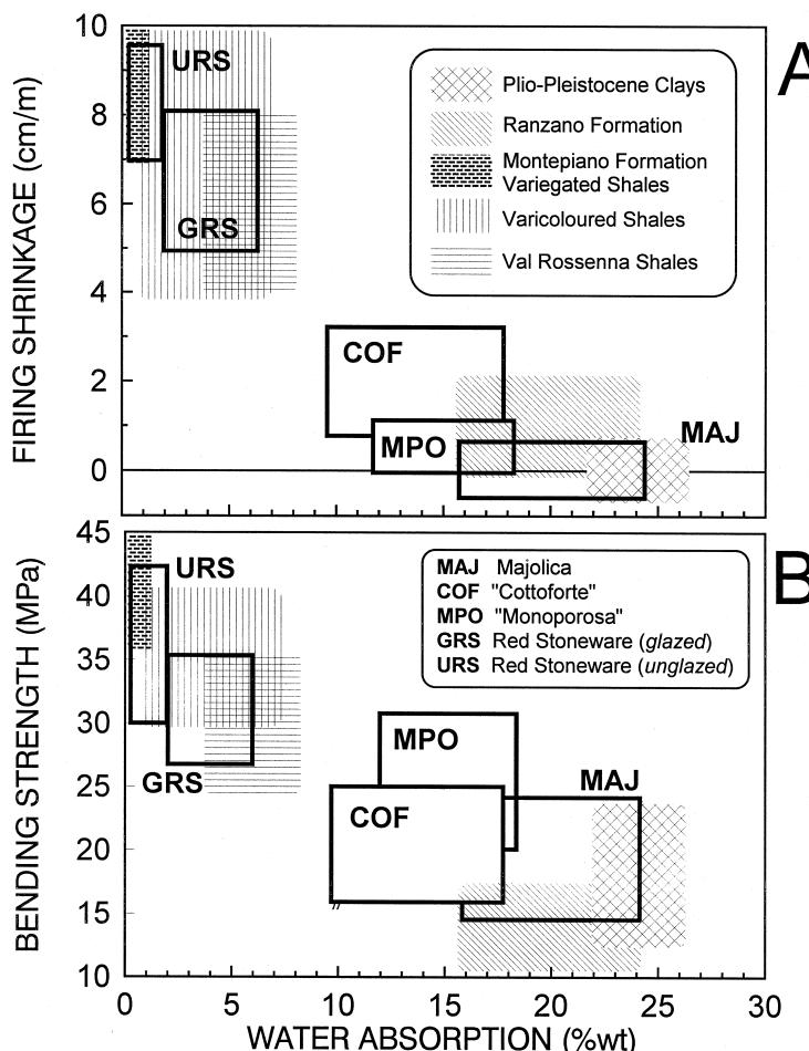
Fig. 10. Technological properties of the products obtained with clay materials from the Sassuolo District in comparison with the requirements of the various types of ceramic tiles. Water absorption versus firing shrinkage (A) and bending strength (B). MAJ: majolica, COF: "cottoforte", MPO: "monoporosa", GRS: glazed red stoneware, URS: unglazed red stoneware.
