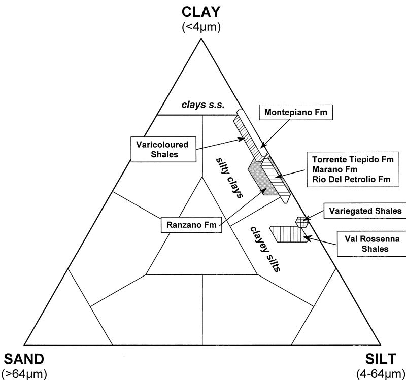
Fig. 5. Ternary diagram (Shepard, 1954) of the grain size distribution of clay materials from the Sassuolo District. Fields represent average  $\pm$  standard deviation of data.
