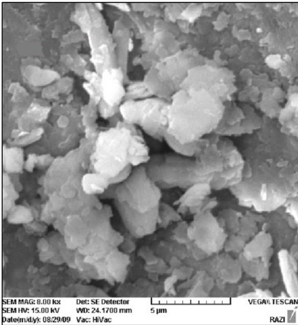
Figure 3. SEM photomicrograph of U1 ball clay sample which shows platelet particles of kaolinite and illite minerals
