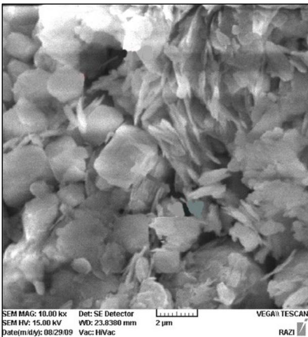
Figure 4. SEM photomicrograph of ARK-10 ball clay sample which shows platelet particles of kaolinite and illite minerals
