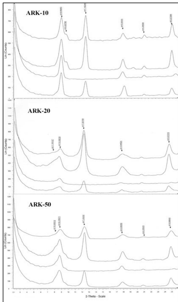
Figure 2. X-ray diffraction patterns of the studied ball clays
