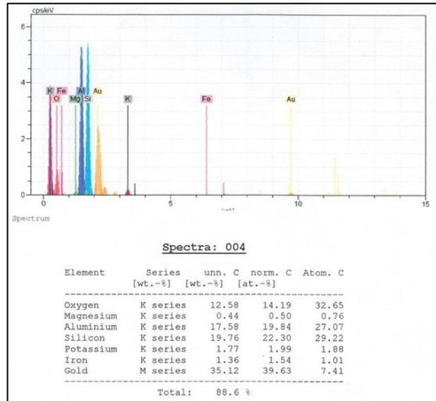
Fig. 5. EDS analysis of kaolinite
