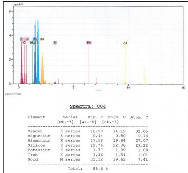
Fig. 5. EDS analysis of kaolinite
