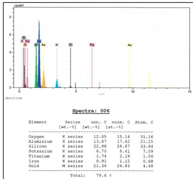
Fig. 6. EDS analysis of illite
